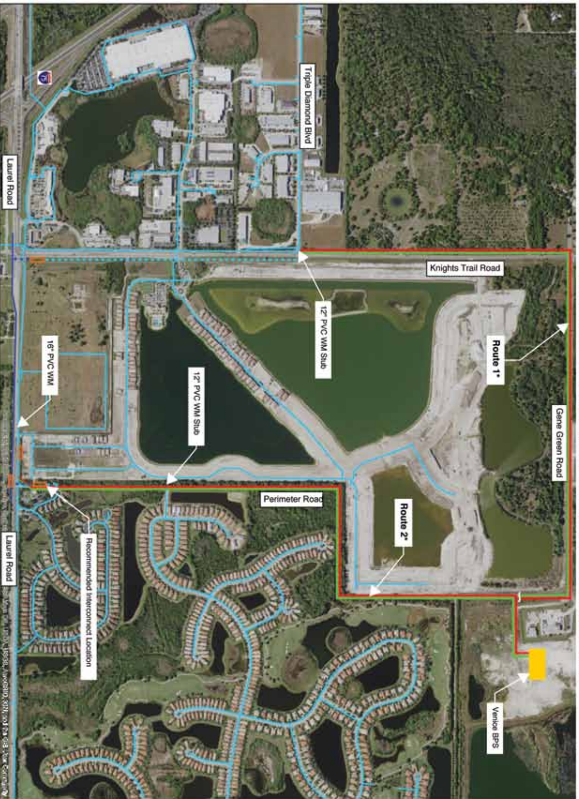
FIGURE 1 - ALTERNATIVE PIPELINE ROUTES AND EMERGENCY INTERCONNECT LOCATIONS
